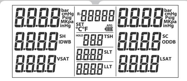
Pressure (bar) bar Psig Pressure (pounds/in<sup>2</sup>) Pressure (kilopascals or N MkPa inHg Negative Pressure (inches Negative Pressure (cm of cmHg SLT Suction Line Temperatur LLT Liquid Line Temperature VSAT Vapor Saturation Temper Liquid Saturation Temper LSAT
